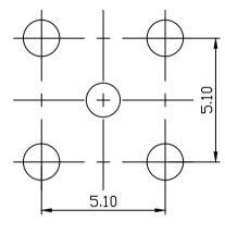
(4) Ø1.5 MIN. (1) Ø1.4 MIN. MOUNTING HOLE
